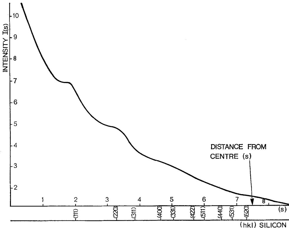
Figure 12 Photometer trace of the amorphous ring patterns in fig. 10. I(s) is the relative scattered intensity at s , where s = (4\pi/\lambda) \sin\theta and \theta is the scattering angle. The (hkl) values show the s values at which rings from polycrystalline silicon would occur.
